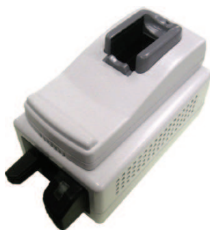
Fig. 6.10. Finger vein enrolment device: a smartcard reader/writer is attached to an FV device. Encrypted finger vein biometric data are securely recorded onto a smartcard onsite so that it can be easily issued to the end-users.
