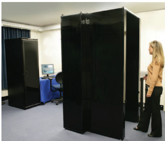
Fig. 7.10. Iris on the Move TM portal: the rack at the far left has the computer, power supplies, and cameras. The portal contains the illuminators which take up a small fraction of its volume. Most of the portal is devoted to guiding the path of the subject and blocking distractions.
