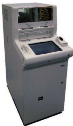
Fig. 6.9. Automated teller machine with FV device: the world's first ATM equipped with finger vein biometrics "AK-1" was released in 2004 and approximately 30,000 units were in operation in Japan as of November 2006.
