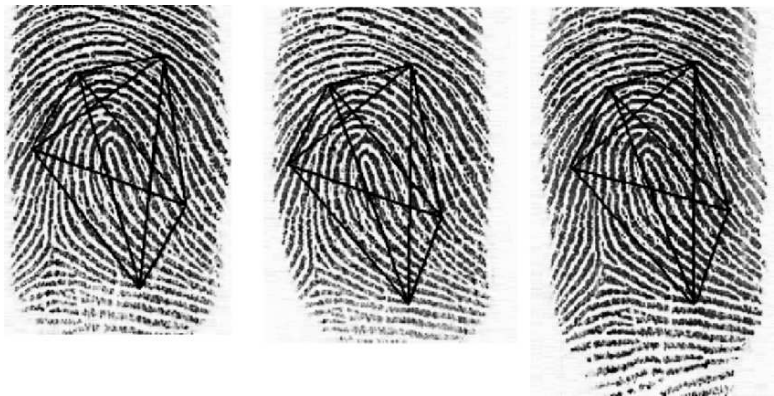
Fig. 3.6. Three reconstructed images of an index finger. Five minutia-points and the ten pairwise distances between them are illustrated by graphs overlaid on the original images.
