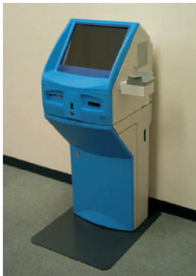
Fig. 5.7. Information kiosk terminal with palm vein authentication sensor unit.
