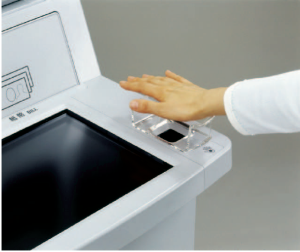
Fig. 5.6. ATM with palm vein authentication sensor unit.
